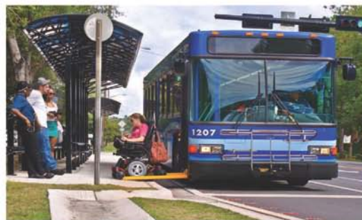
A "Smart Bus" bay located on Southwest 20th Avenue in Gainesville enables buses to load and unload riders without impeding through traffic.
