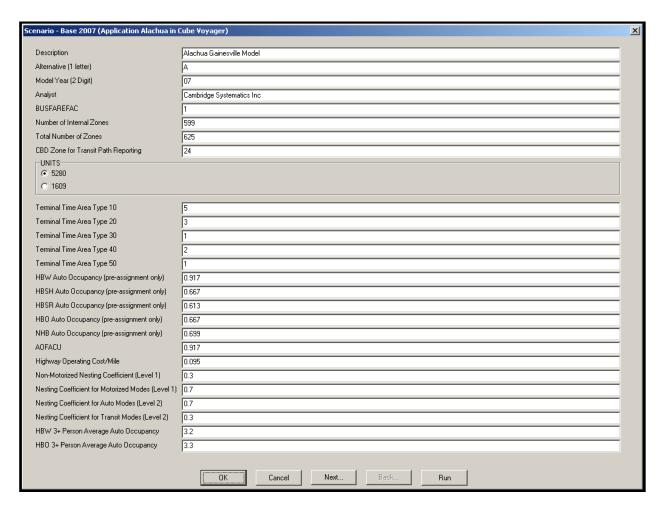
This dialog box allows you to change model runtime options and set model parameters. These parameters are stores as Cube Catalog Keys which are effectively variables which are references in the model script during the relevant model processing phase. The Catalog Key values can also be observed in Part 4 of the Catalog File diagram above.
