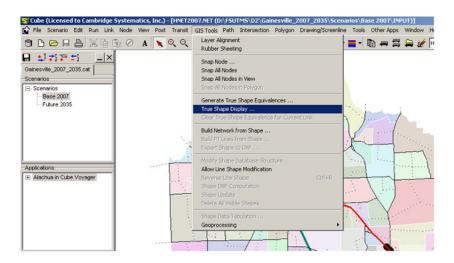
Step 3 "A" should be selected for A-Node, "B" for B-Node and "N" for Node Number. Click Ok.
