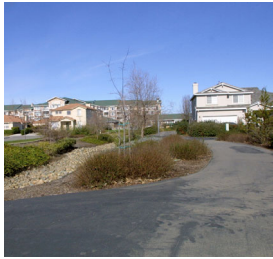
Pedestrian / cycle link between neighborhoods with integrated stormwater catchment swale. Davis, California
